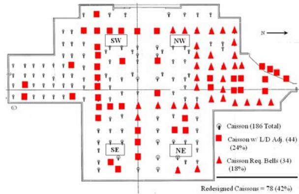
Figure 9 – Summary of Impacted Drilled Shafts
