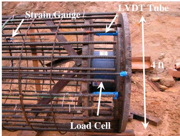
Figure 8 – Drilled Shaft Load Test
