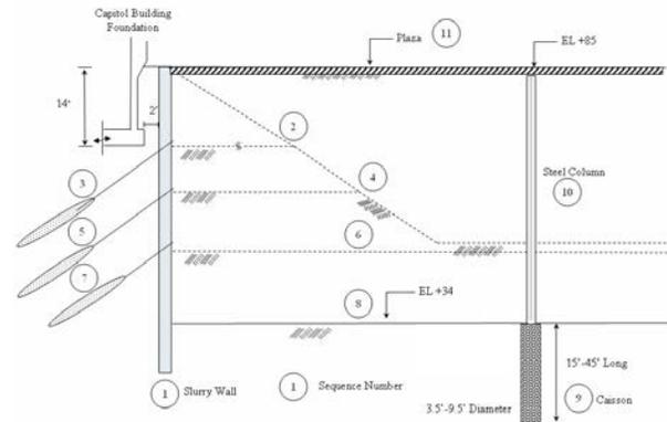
Figure 2 – Actual Construction Sequence
