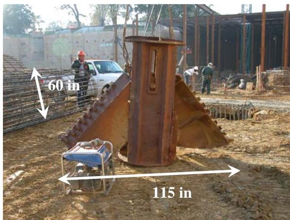
Figure 11– Drilled Shaft Belling Tool
